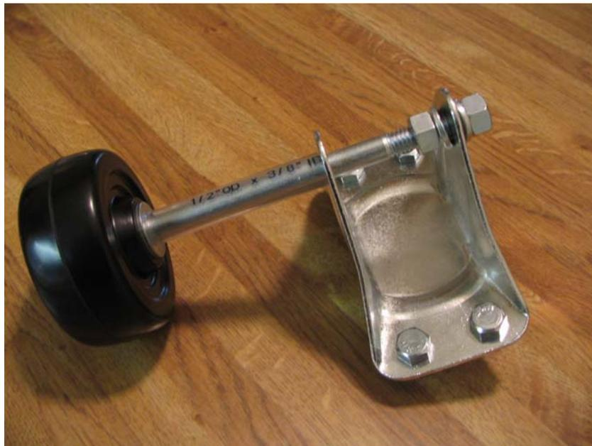
Figure 4. Guide Wheel Assembly
